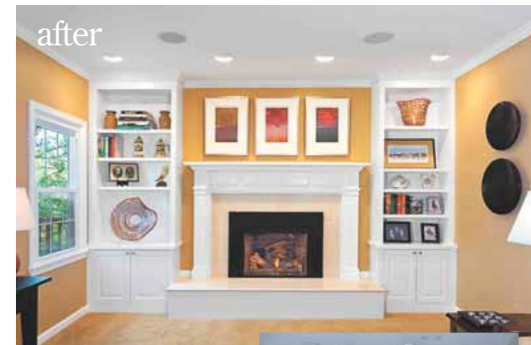
The existing half-brick floor-to-ceiling backwall was replaced by perfectly symmetrical built-ins, crown molding and an elevated hearth with a marble surround and Edwardian-style mantle.
